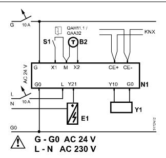
N1 Room thermostat RDU341 V1 Damper actuator, VAV compact
