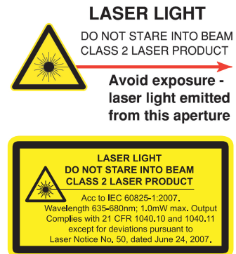
Figure 2. FDA (CDRH) warning label (Class 2)
