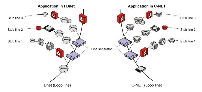
The line separator can be integrated in the supply shaft on every floor in an intermediate distribution frame, or at the place of the collective control unit. When all stubs are guided individually to the collective control unit, insert the line separator directly in the new fire detection control unit.
