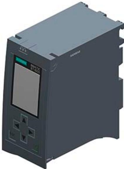
SIMATIC S7-1500, CPU 1515-2 PN, CENTRAL PROCESSING UNIT WITH WORKING MEMORY 500 KB FOR PROGRAM AND 3 MB FOR DATA, 1. INTERFACE: PROFINET IRT WITH 2 PORT SWITCH, 2. INTERFACE: ETHERNET, 30 NS BIT-PERFORMANCE, SIMATIC MEMORY CARD NECESSARY
