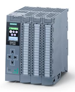
SIMATIC S7-1500 COMPACT CPU CPU 1512C-1 PN, CENTRAL PROCESSING UNIT WITH WORKING MEMORY 250 KB FOR PROGRAM AND 1 MB FOR DATA, 32 DIGITAL INPUTS, 32 DIGITAL OUTPUTS, 5 ANALOG INPUTS, 2 ANALOG OUTPUTS, 6 HIGH SPEED COUNTERS, 1. INTERFACE: PROFINET IRT WITH 2 PORT SWITCH, 48 NS BIT-PERFORMANCE, INCL.FRONT CONNECTOR, SIMATIC MEMORY CARD NECESSARY
