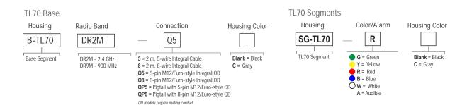
Select the 5-pin base for tower light configurations of up to three modules. Select the 8-pin base for tower light configurations of up to six modules, or when the event counter will be enabled.
