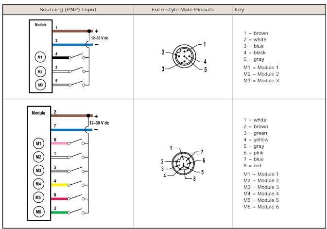
Input wires M1 through M6 can be used to either control the light segments or can be configured as external PNP Inputs. Refer to the DIP switch settings for configuration instructions.
